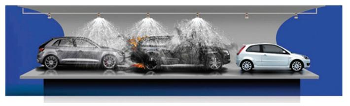
Third scenario of using ECS is a pre-programmed system, when a fire signal from the first activated sprinkler or from a fire detector activates the sprinklers not only in the area of a fire but on the way of its spread. For example, preventing of flame spread through the doorways and windows in hotels or offices is crucial in high rise buildings.
