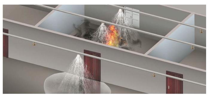
A proposed technology uses an electrical activation, so there is no necessity to install sprinklers on the ceiling. They can be oriented in such way that will ensure maximum efficiency of the fire extinguishing.
