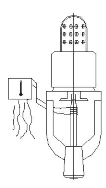
The second improvement introduced in this work is the facility to monitor the activation of the sprinkler. Such a facility consists of the interrupting contact placed between the bulb and the lock valve. The contact is closed when sprinkler is inactive and it disconnects when the sprinkler activates. Availability of the check-up facility is crucial for getting information of sprinkler status. It may be used when we need information about precise location of fire.
