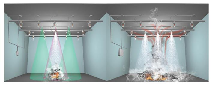
The lower calorific power of a fire source at the moment of activation allows reducing the amount of water required for fire extinguishing. In many cases it's a very important advantage. Also it helps to decrease the size of pipes, the power of pumps and the volume of reservoirs.
